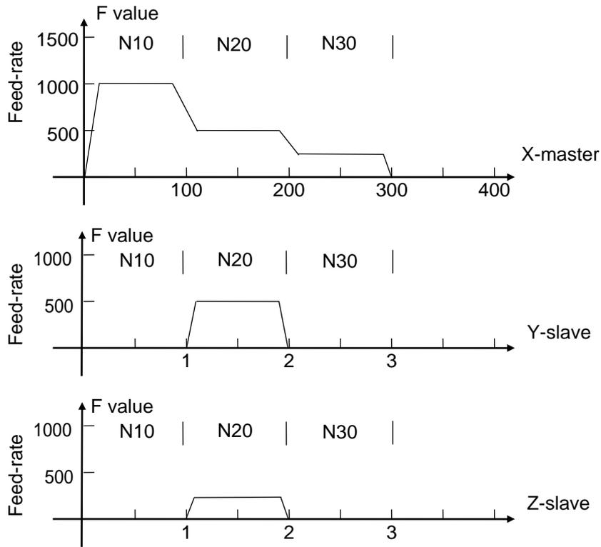
Fig 3-4 Master/ Slave Mode - linear Acc./Dec.
