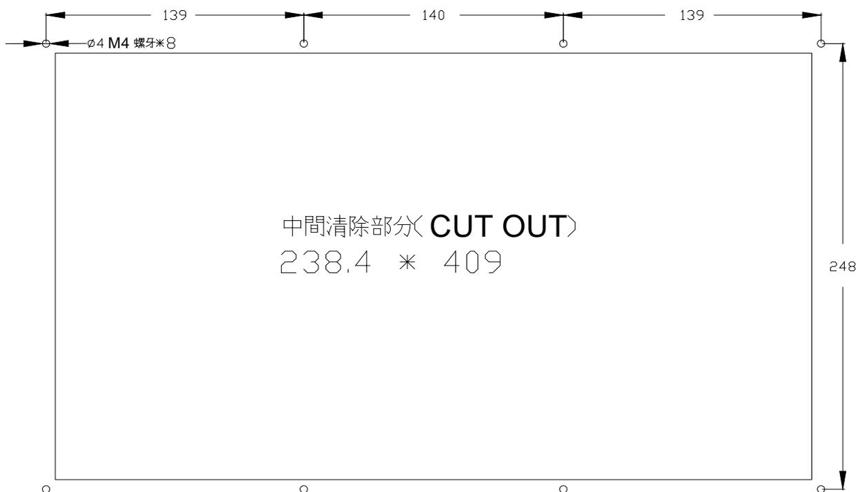
Fig. 5-6 Control Unit Cutout Dimensions
