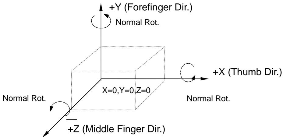
Fig 2-24 3-D Coordinate System (Horizontal Milling Machine)
