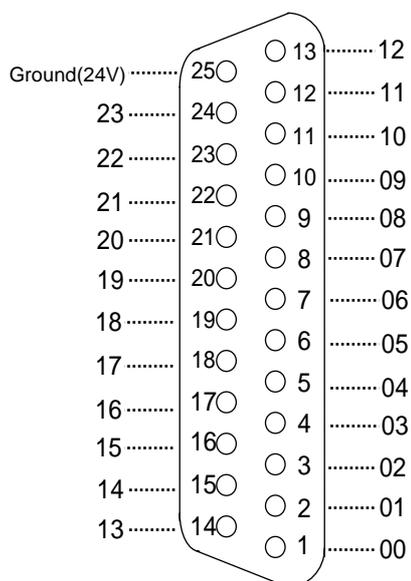
Pin assignment (Output) of H4CL-M P1 (male) connector
