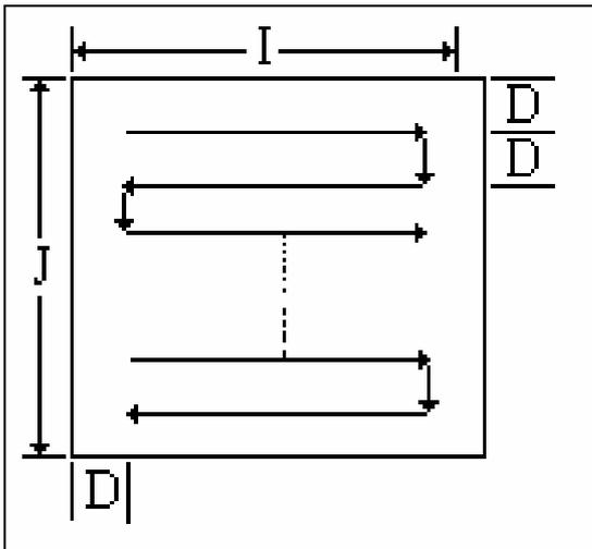
As shown in the above figure, an inner square is cut in a S-shaped groove-milling manner. Then cut again along the side to remove the part that is not cut during the S-shaped groove milling process.
