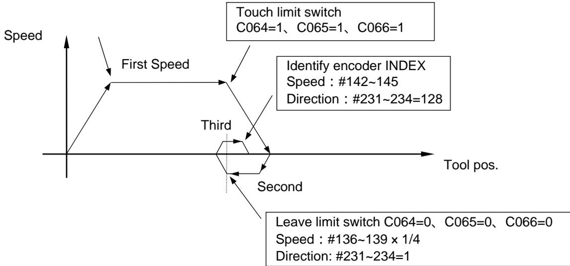
Fig 4-2 (B) Homing Speed and Homing Grid Direction
