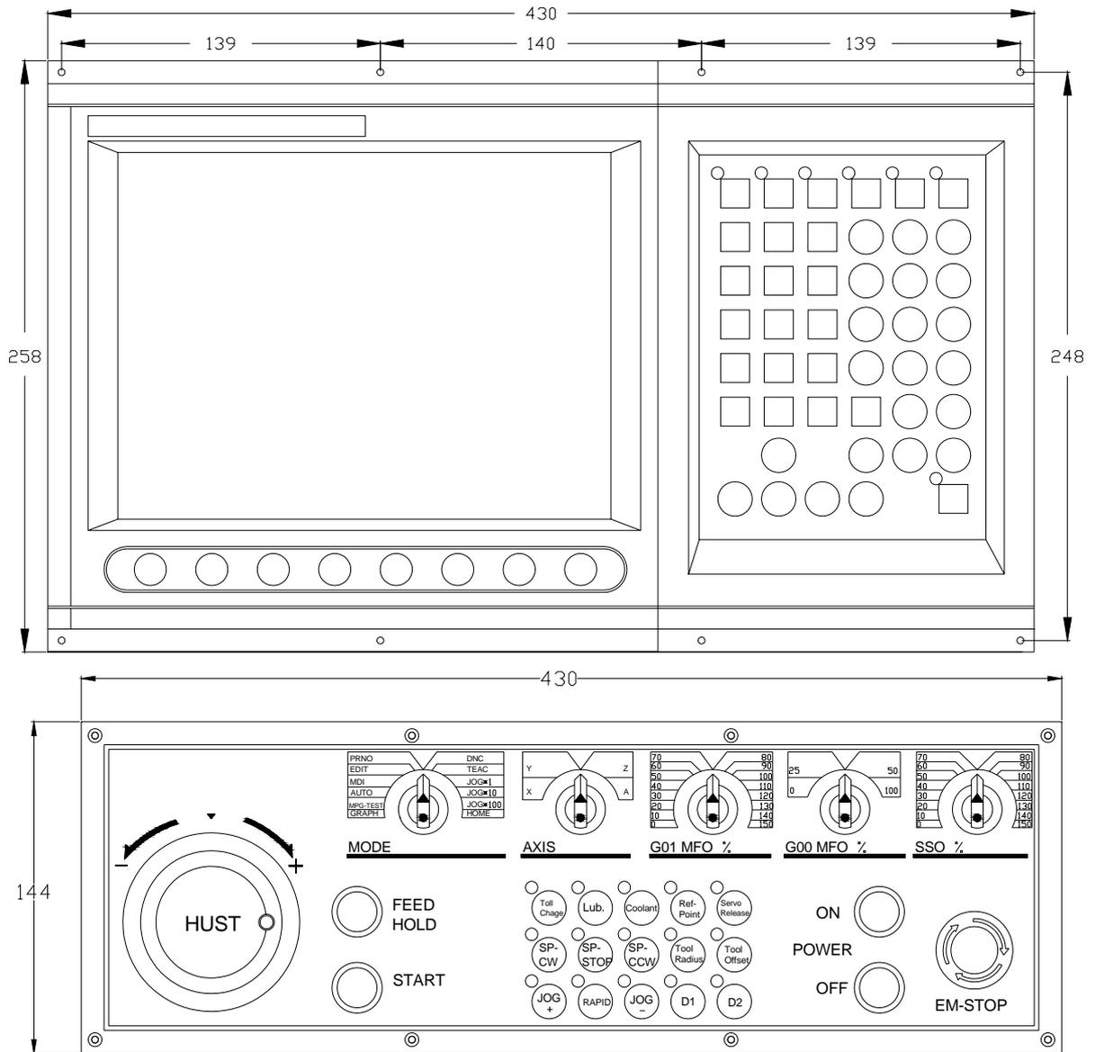
Fig. 5-4 H4CL-M Series Control Unit Case Dimensions
