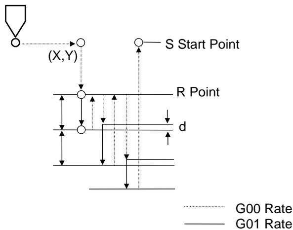
Fig 3-42 G83 Deep Drilling Canned (peck drill) Cycle
