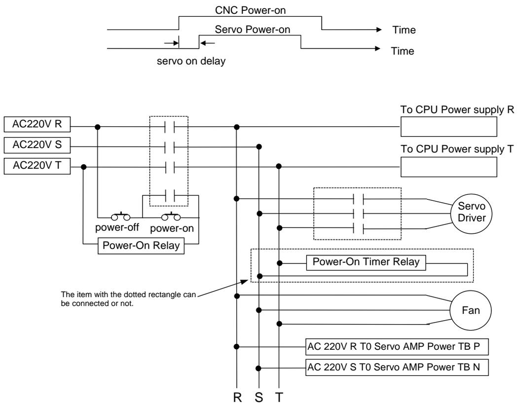
Fig. 5-26 System AC Power Connection
