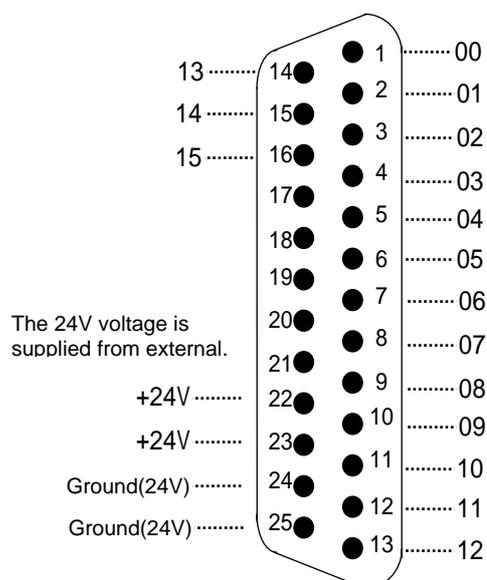
Fig. 5-12 I/O Connector Pin Assignment (NPN-type)
