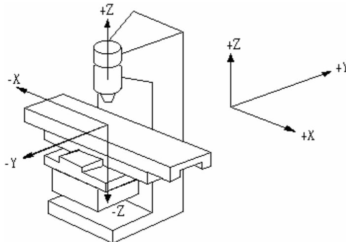
Fig 2-25 3-D Coordinate System (Vertical Milling Machine)
