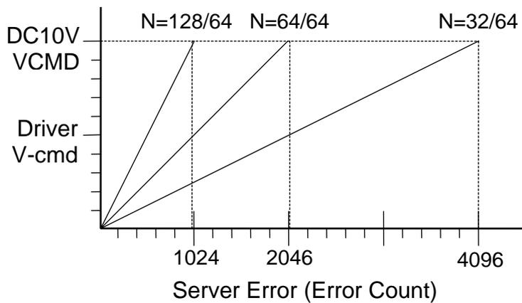
Fig 4-4 Relationship between the Driver V-command and Servo Error
