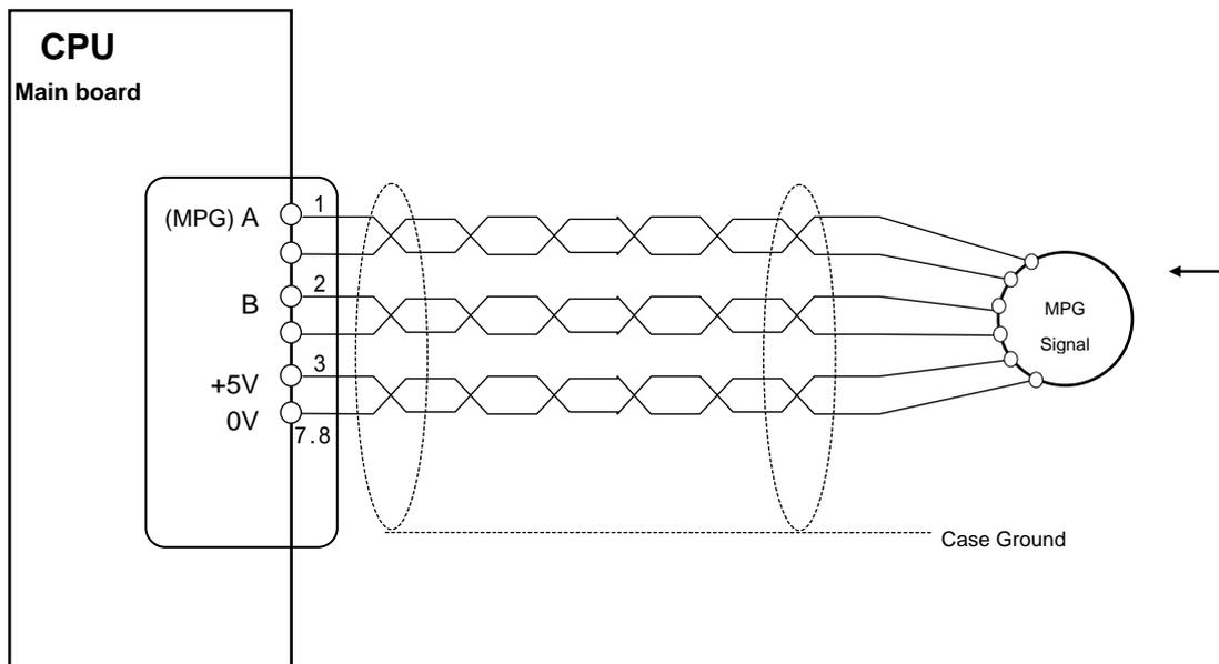
Fig. 5-25 Axes, Spindle, and MPG connection
