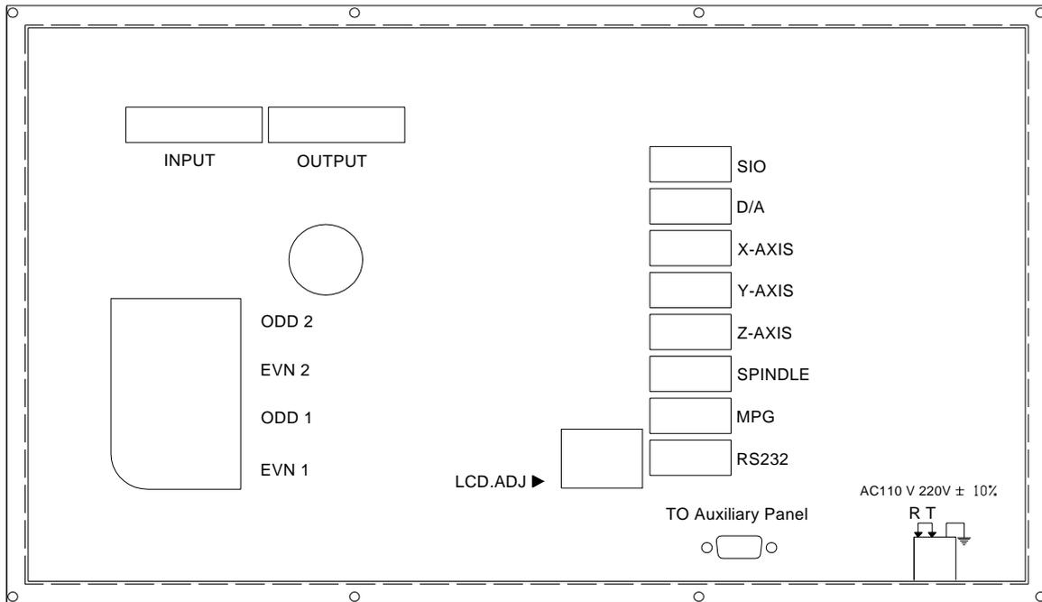
Fig. 5-3 H4CL-M CPU Main board Connectors
