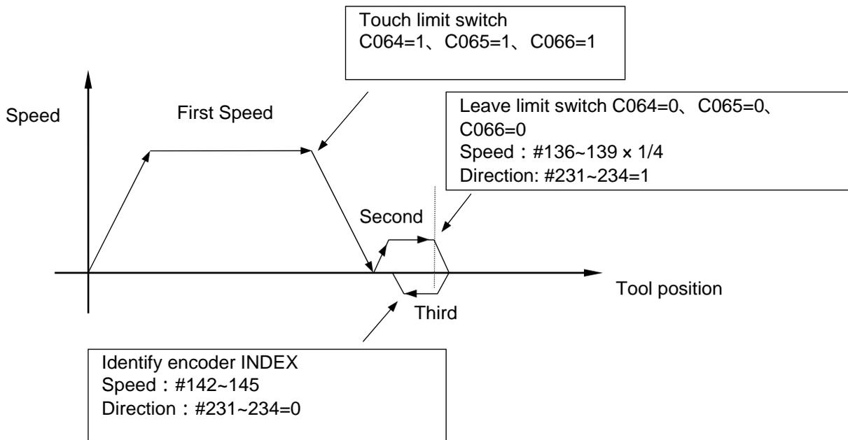
Fig 4-2 (C) Homing Speed and Homing Grid Direction
