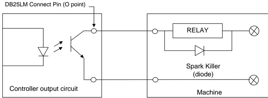
Fig. 5-15 Output Line (without the output relay board)
