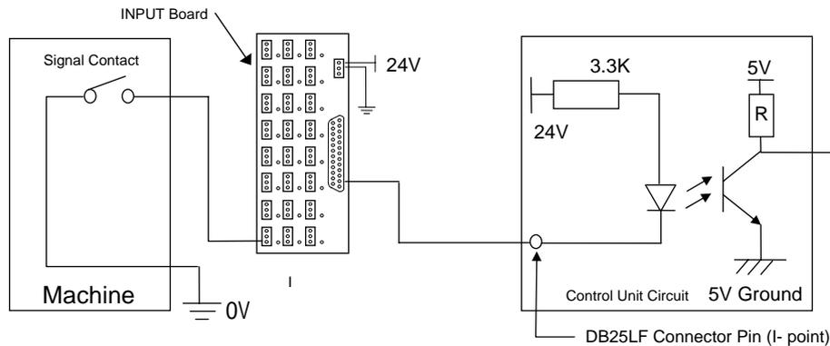
Fig. 5-14 Input Signal Connection (input to the control unit via the input board)
