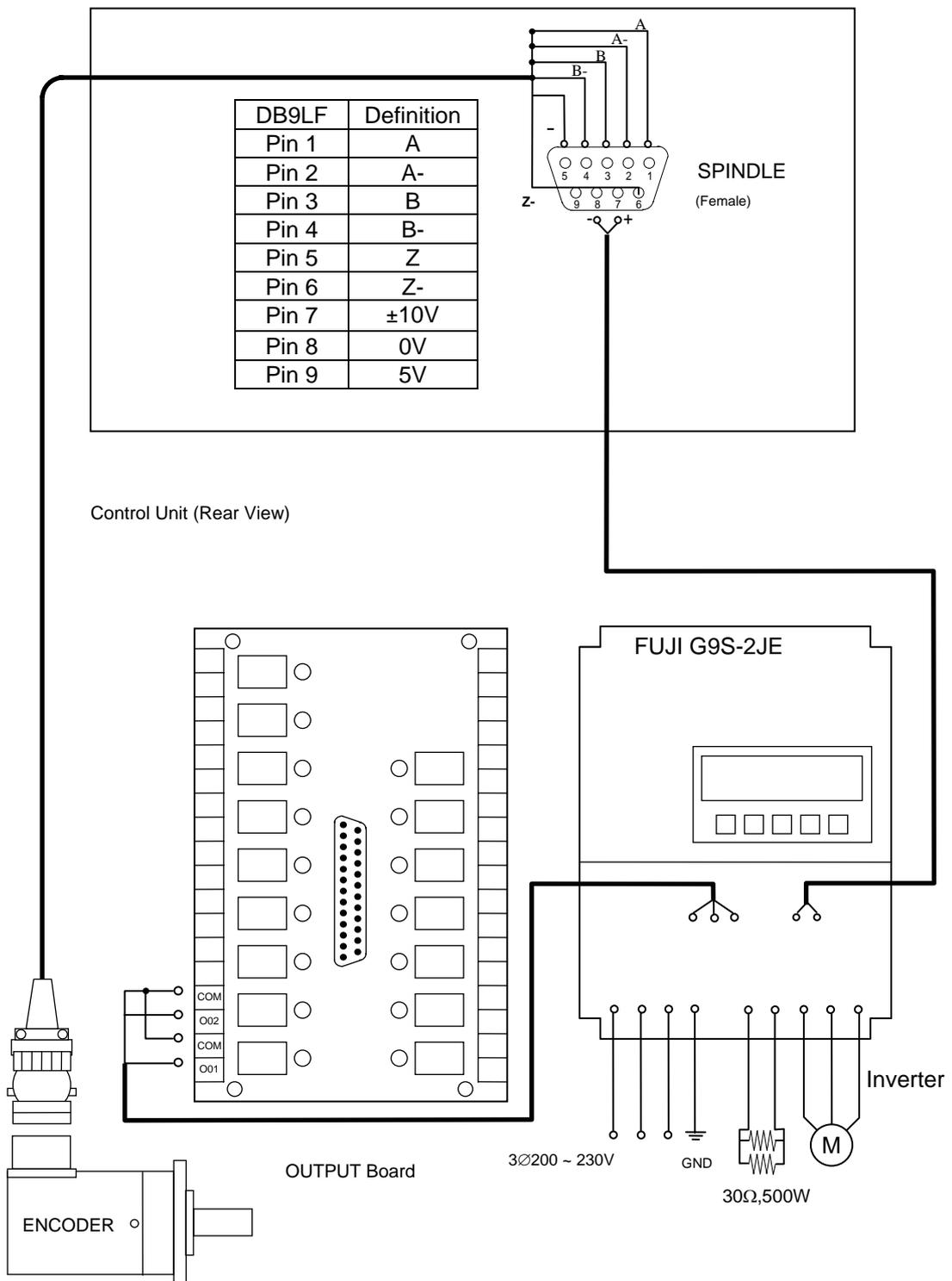
Note: It is recommended to connect 24V for the contacts on the output board.
